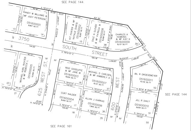
7' UTILITY & DRAINAGE EASEMENTS EACH SIDE OF PROPERTY LINES AS INDICATED BY DASHED LINES EXCEPT AS OTHERWISE SHOWN.
